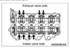
Measure the valve clearance. If the valve clearance is not as specified, loosen the rocker arm lock nut and adjust the clearance using a thickness gauge between the camshaft and the roller while turning the adjusting screw. Standard value (cold engine): Intake valve: 0.09 mm Exhaust valve: 0.14 mm
