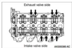
10.Measure the valve clearances at the places indicated by arrows in the illustration. If the clearance is not within the standard value, repeat steps 7 and 8 above.
