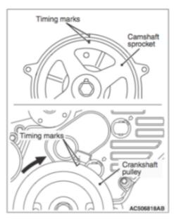
Align the camshaft sprocket timing marks and set the No. 1 cylinder at top dead centre.
