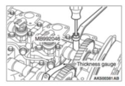
While holding the adjusting screw with a screwdriver to prevent it from turning, tighten the lock nut to the specified torque using a valve adjusting socket. (MB992046)
